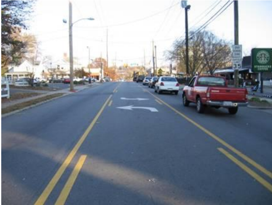
Figure 5.4 Two Way Left Turn Lane
